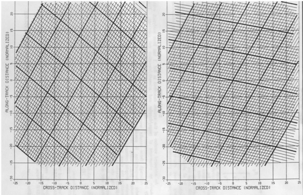
**Azimuth-Elevation (FLIR) Map Coordinate Loci**
